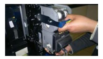
Removing the chassis from the housing.
